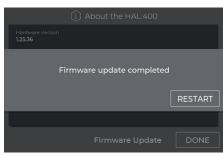
After completing the download, the HAL:400 will load the new firmware automatically. Upon completion the HAL:400 will require a restart in order to apply the updates.
