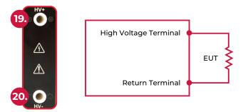
Connect the (Red) High Voltage test lead to the High Voltage Terminal (19) and ensure the plug is firmly connected into the socket.
