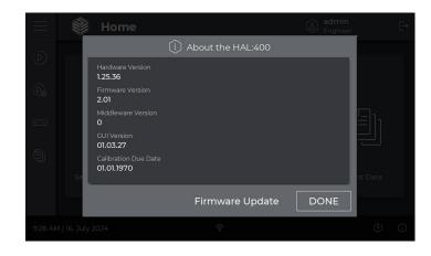
The resulting screen, above displays useful information about your HAL:400 including the hardware version, firmware versions. In addition a reminder function for the calibration due date will also be displayed.
